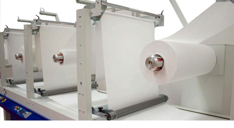
The RF Line is a modular cutting system that can be equipped with a different number of feeders and with different die cutting punches depending on specific customer requirements. The main benefits are:
