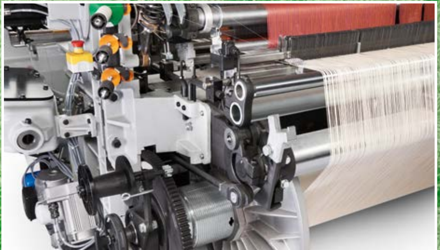
Best-in-class Loop Formation: New Ground Back-Rest Roller
