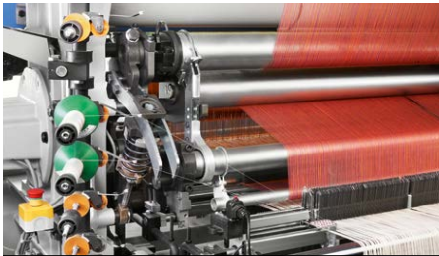
Best-in-class Loop Formation: New Positive Pile Back-Rest Roller
