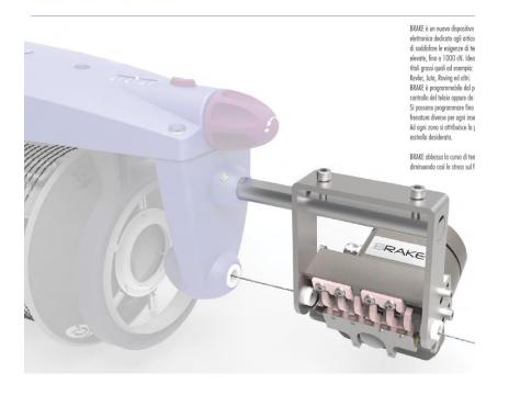
BRAKE is a new electronic braking device dedicated to technical textiles, that is able to meet the needs of very high tension, up to 1000 cN. It's ideal for yarns with coarse counts such as for example: Flat Tapes, Chenille, Kevlar, Jute, Roving and more.
