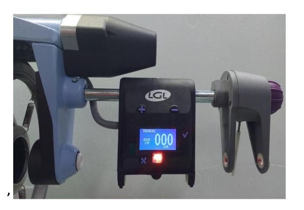
The new electronic brake keeps the output tension constant.
