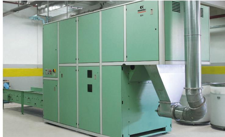
The B15 at the exit can also be equipped with an opening unit, the B18. This is the ideal solution to process small lots of already-cleaned material to feed one or two cards.
