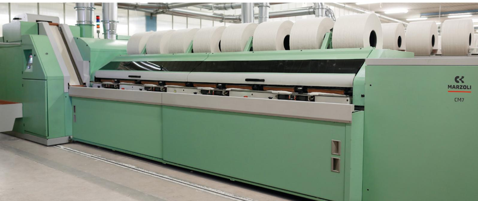
Comber with 8 combing heads, automatic can change and automatic lap piecing technology (option). Thanks to the variable speed of the circular comb and the revised kinematics of the nipper the machine can reach up to 600 nips per minute, enabling production levels up to 85 kg/h.
