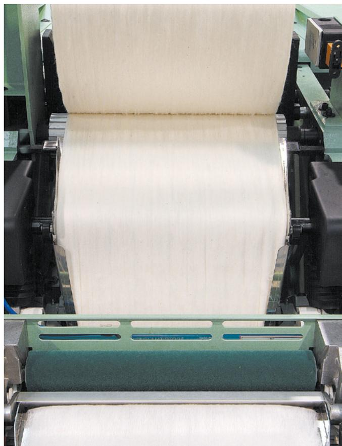
Standing pendulum movement of the nipper to maintain minimum and constant distance between the jaws and the circular comb throughout the combing cycle. Top quality of circular combs with 4 sectors (combing angle of 90°) or 5 sectors (combing angle of 112°) with progressive point density, specifically designed to process thick batts at high speed.
