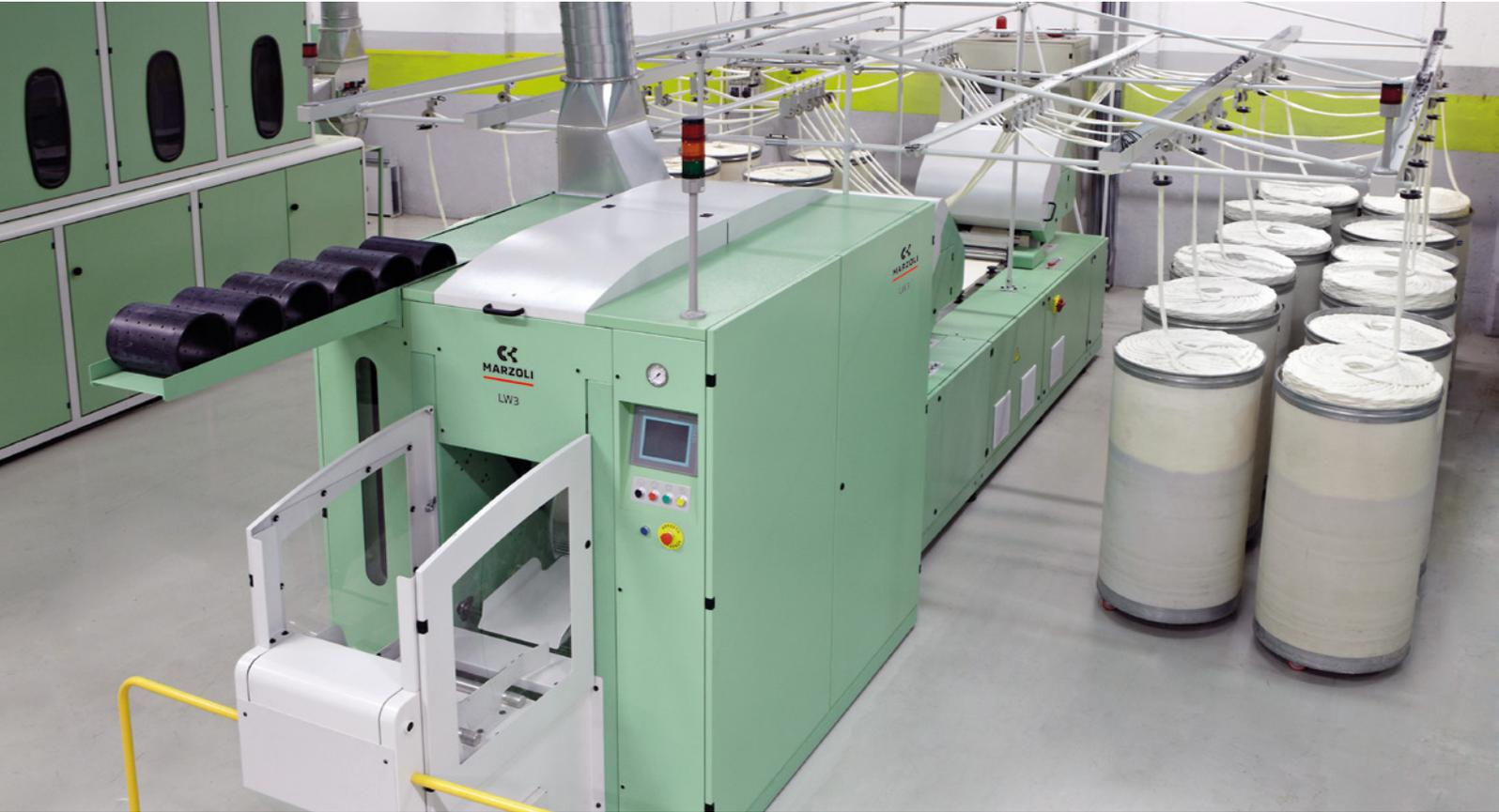
The LW3 lap winder represents the best technology for quality and productivity. The innovative design of its lap formation area with 4 calenders and a compacting cylinder to avoid expansion of the wound layers allows to reach an average speed of 190 m/min. This, together with an automatic doffing system of only twenty seconds,
