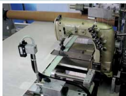
Mod. R12-4C Crochetta automatica Automatic fagoting and picoetta edging
