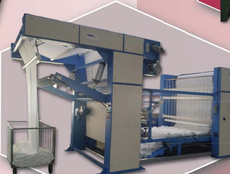
Uscita combinata grande rotolo / falda Combined exit Aframe / plait
