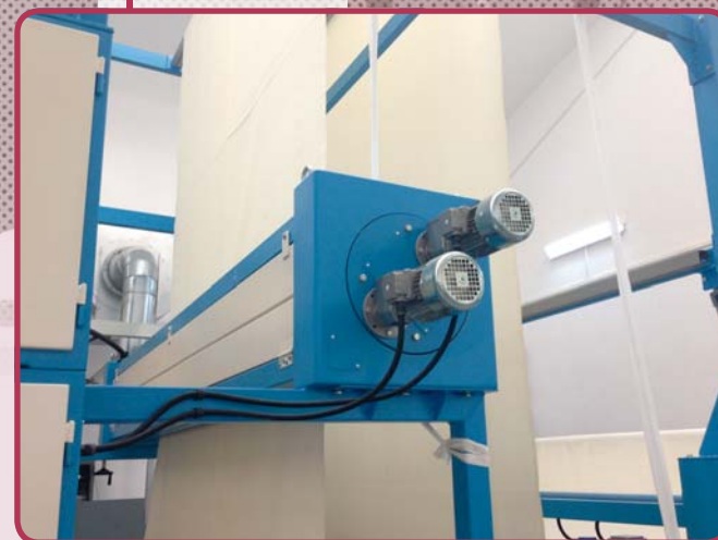
Spazzole combinate a settori Combined brushes with sectors
