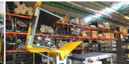
EV80/90 Tilting platform for metal containers
