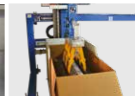
Handling device for unloading in cardboard boxes
