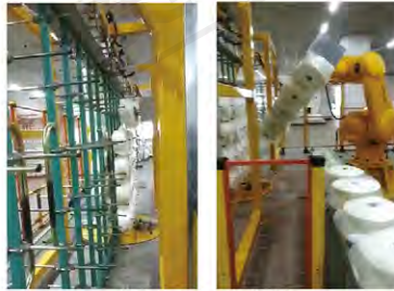
机械手自动换纱 Manipulator to change the yarns automatically
