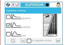
Allows the choice of different regulation conditions according to fabric requirement
