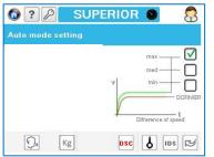
Batching unit speed fully synchronized with weaving machine
