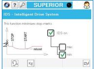
Selection of different tension conditions during halt to avoid stop marks
